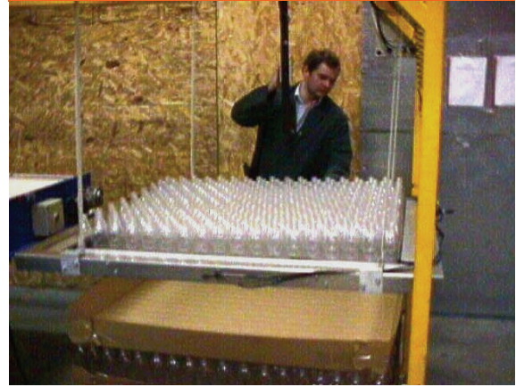
LAYER LOWERED ONTO PALLET
