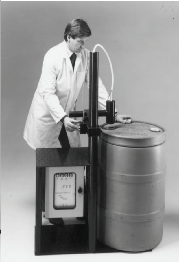
One tester—two different applications. Simple dual purpose frame. This picture shows an 'old style' model. Operator control panel of new electronics are mounted on the vertical pole.
