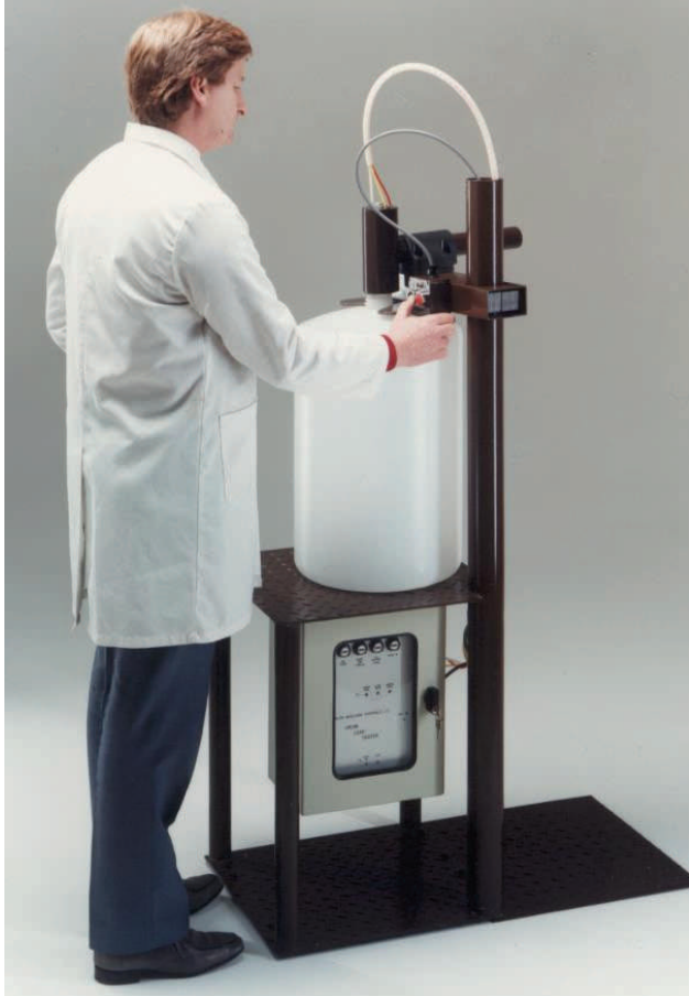
One tester—two different applications. Simple dual purpose frame. This picture shows an 'old style' model. Operator control panel of new electronics are mounted on the vertical pole.
