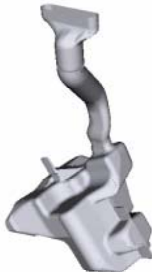
Figure 7. Geometry of the windshield washer fluid reservoir
