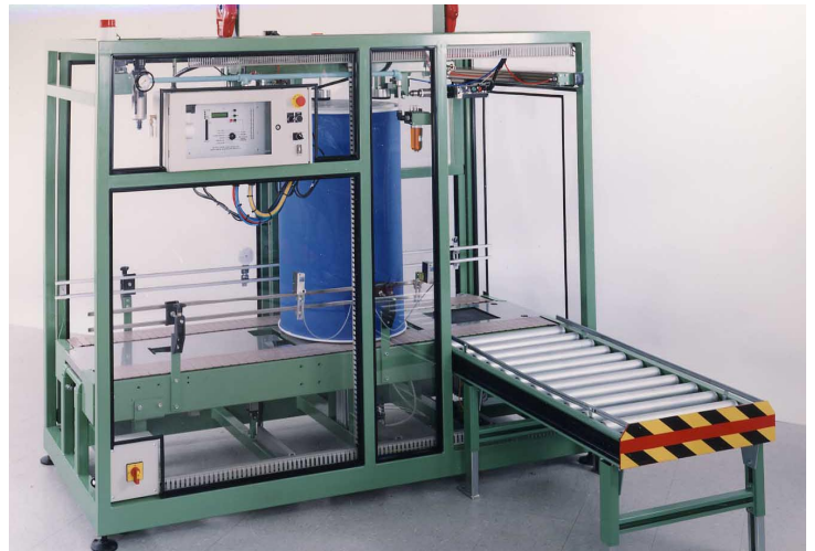
Automatic drilling, container weighing, leak testing, data logging, and patented feedback weight correction to parison programmer — Standard features, Temperature compensation next !
